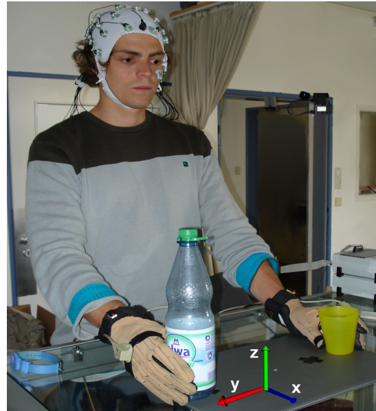
Fig. 1. A subject wearing EEG cap and sensor gloves during the experiment. The directions of the coordinate axes are illustrated.
