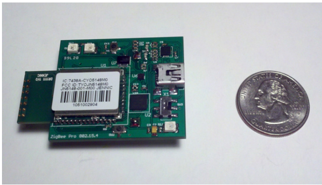
Fig. 1. Sensor board for the Slips and Falls Predictor prototype.
