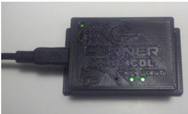
Fig. 2. ABS plastic case for the Slips and Falls Predictor, with a USB cable connected to the board.
