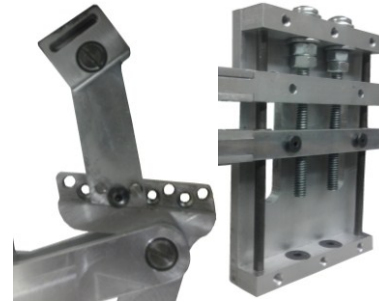
Figure 2. Finger size adjustment of the proximal phalanx (left) and vertical adjustment of the 8-bar mechanisms for the middle and index fingers (right).
