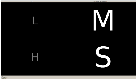
Fig. 1: P300 visualization is divided into four states: Low-speed, Medium-speed, High-speed and Stop. A fifth state is detected by the system when the user is not looking at the screen.
