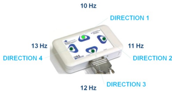
Figure 2. The g.SSVEP box used to present stimuli. Each of the four LEDs flickered at a different frequency from 10-13 Hz.
