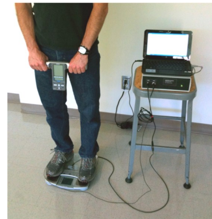
Figure 1. Left: illustration of the BCG/ECG system deployed in clinic. The signal conditioning box is powered through the isolated USB. Right: picture of the whole system, with a test subject standing on the BCG scale and holding the two-electrode, handlebar ECG.
