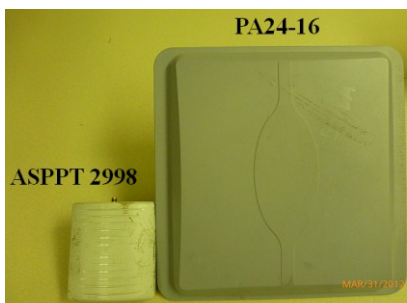
Fig. 1. A photograph showing a comparison between physical size of PA24-16 (29 x 29 x 2.5 cm 3 ) and ASPPT 2998 (10.5 x 10 x 4 cm 3 ).
