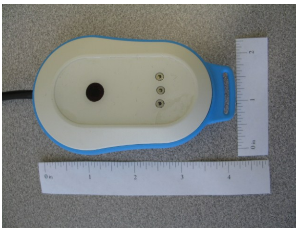
Figure 1: CW-NIRS probe using 3 laser diodes (680nm, 830nm, 980nm) and one photodetector with NIR optical filter. The distance between sources and detector is 30mm.
