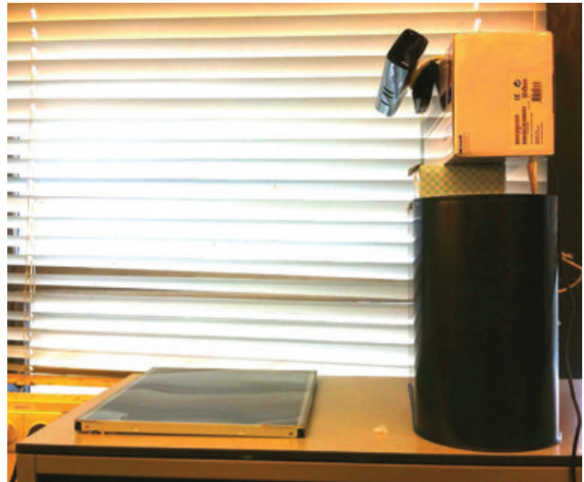
Fig. 3. The Xbox Kinect together with the NecTouch software is used to turn a normal screen into a (significantly larger) multi-touch screen
