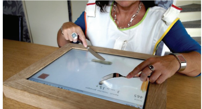
Fig. 1. Task oriented training of dining skills using actual knife and fork, to play the game on a pressure sensitive touchscreen device. The patient wears the motion sensing jacket that is used for providing graphical and vibrotactile feedback regarding posture and to influence directly the game play
