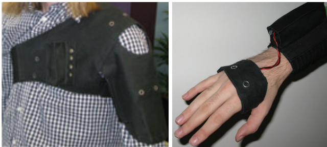
Fig. 2. Improved Sensor Vest and Sensor Glove for tracking hand movement
