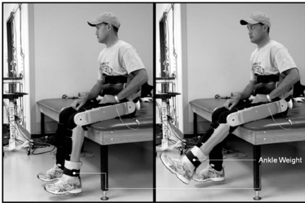
Figure 2. Experimental setup for cooperative control of weighted leg lifts.
