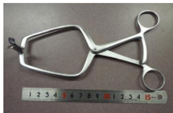
Figure 3. Small size retractor employed to simulate the arching spine
