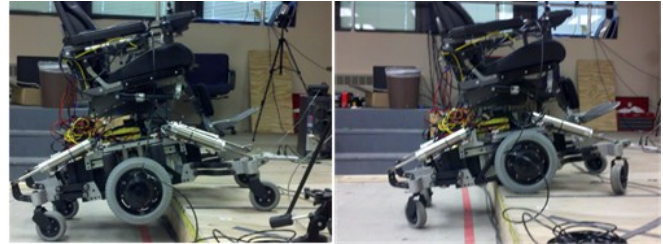
Figure 5 Gen II PerMMA in automatic climbing mode
