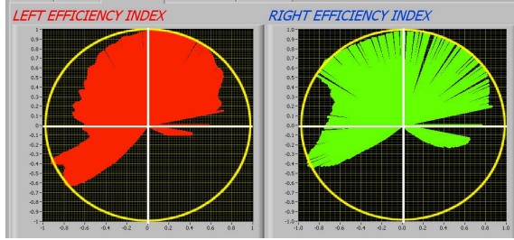
Figure 1: Visual feedback of the instantaneous mechanical efficiency, based on a polar plot diagram where each line has amplitude proportional to the instantaneous mechanical efficiency and phase proportional to the pedal angle. If the circle is entirely filled (red for left pedal and green for right pedal), then IE equals 1. The polar representation communicates also the information related to the different phases of the pedaling cycle with the associated theoretical optimal pedaling strategies. In this way the efficiency is directly related to each part of the cycling revolution.
