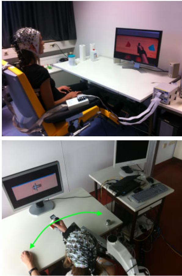
Fig. 2. In the first session (top), the user was asked to move a virtual arm in a screen that simulated the selection of two targets (left/right). In the second session (bottom) the arm not involved in MI was controlled directly by the classifier output using the ArmeoSpring. The green line depicts the trajectory of the neuroprosthesis.
