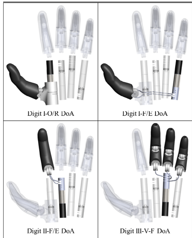
Fig. 1. Degrees of freedom corresponding to each degree of actuation (Note that O/R refers to Opposition/Reposition, F/E refers to Flexion/Extension, and Digits III-V are only actuated in Flexion).
