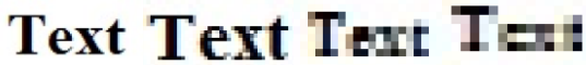
Figure 1. The word “Text” at five degrees of pixelization. (a): 80×40 pixels. (b) 40×20 pixels. (c) 20×10 pixels. (d) 16×8 pixels.
