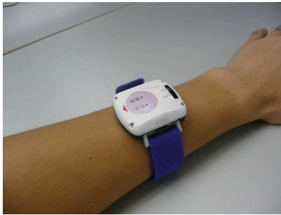
Fig. 7. Wrist-type Photoplethysmography sensor in this study (Acceleration sensor is also built in)
