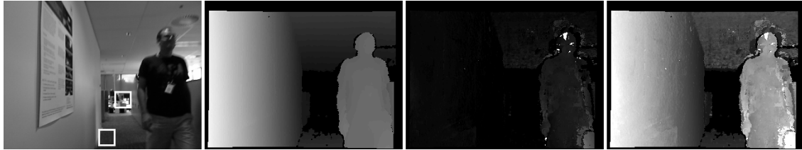
Fig. 2. From left to right: (a) original images (boxes show static- and moving-object measurement windows); (b) D_t (depth-based); (c) \tau^{-1} (i.e., time-to-contact response); and (d) V_t ( \tau -based, \lambda = 125 ). Note different locations of poster in Seq. 2 confirming camera motion. Best viewed on screen.
