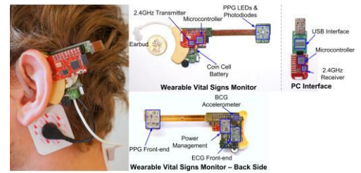
Fig. 4 Left: The wearable vital signs monitor worn at the ear. Center top: Front side of the monitor with MSP430, radio, battery and PPG sensor outlined. Center bottom: Back side of the monitor with PPG and ECG front ends, power management and accelerometer outlined. Right: The USB interface that allows the device to interface with MATLAB.
