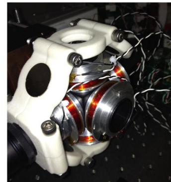
Figure 3. (a) Imaging system schematic. (b) Photograph of the magnetics subsystem and the central imaging chamber.
