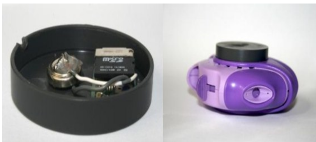
Figure 1: (Left) The adherence monitoring device (Right) The adherence monitoring device bonded onto the side of a Seretide Accuhaler/Diskus inhaler
