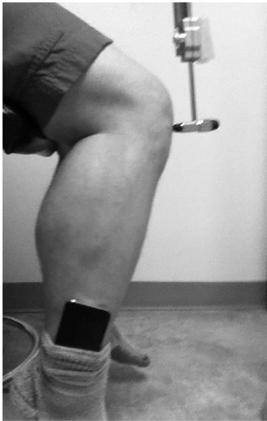
Fig. 1. iPod wireless accelerometer reflex quantification system with iPod wireless accelerometer mounted above and adjacent to the lateral malleolus.
