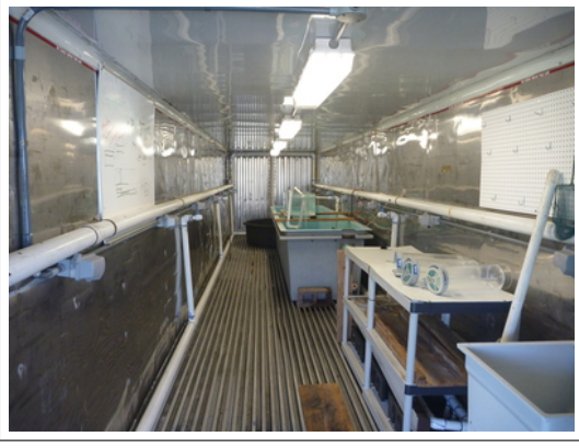
Fig. 2. Interior view of converted shipping container used as testing area for the experiments. This area was located near the tanks used for raising the fish and provided a controlled environment for initial experiments.
