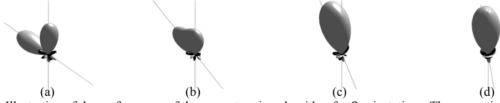
Figure 1: Illustration of the performance of the reconstruction algorithm for 2 orientations. The separation angles are 90 (a), 60 (b), 30 (c) and 10 (d) degrees. In all cases, the orientations are recovered to machine precision.
