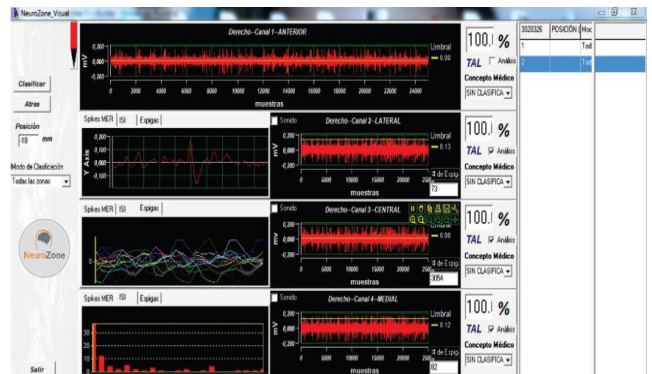
Fig. 5. Operating Room. In this window the specialists observe the signals acquired in real time (5 Channel max.). They can analyze the recordings and label them. The applications for Inter Spike Interval analysis and on-line recognition of brain structures are also available.
