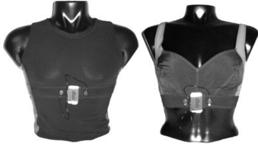
Figure 3. Custom made male base layer and female bra. Each include two textile electrodes, male snaps and a pocket for the Shimmer sensor.
