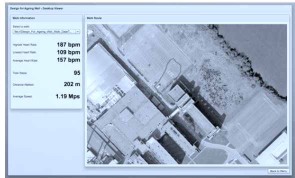
Figure 2. User Interface of the Desktop Viewer software showing an interactive map with recorded data overlaid and health and activity information.
