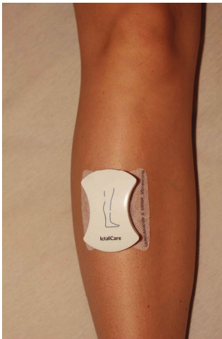
Fig. 1. The wireless sEMG device placed on the tibial muscle.
