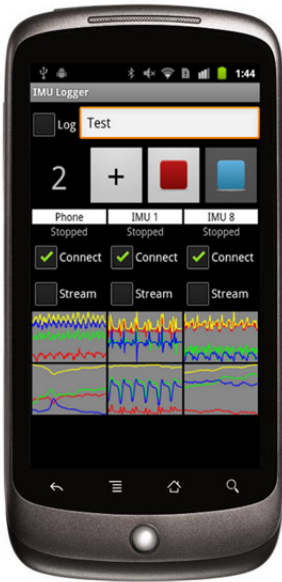
Figure 2: IMU Logger application showing three-axis accelerometer and magnetometer data from the phone and two IMUs.
