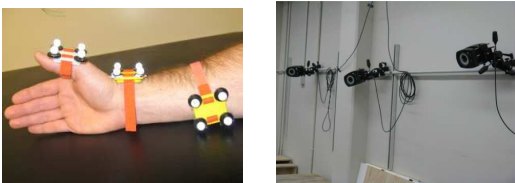
Fig. 1. Markers placed in the thumb and data capture setup
