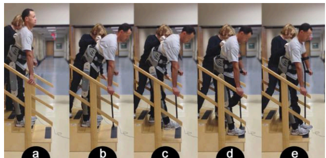
Figure 3. Stair descent sequence, showing a) starting posture, b) leaning forward for CoP trigger, c) extension of right leg over subsequent stair tread, d) lowering of body and right foot to subsequent stair tread, and e) movement of left foot to subsequent stair tread.
