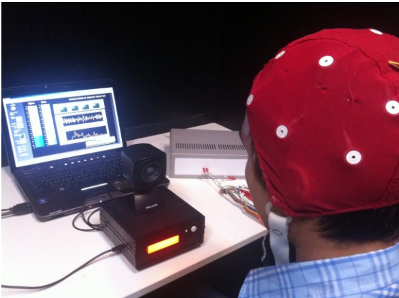
Fig. 3 The proposed SSAEP-based BCI system.
