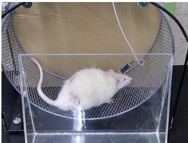
Fig. 6. A wheel to exercise a small animal that we converted into locomotion recorder for a rat.
