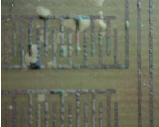
Fig. 6. Optical photograph of an IDE after testing at 85°C showing a defect that led to device failure.
