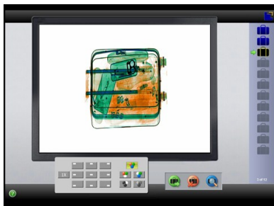
Figure 2. Screenshot of SPI X-ray screening computer-based training software. The software emulates X-ray screening equipment functions, including color filter layers.
