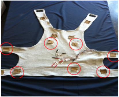
Figure 2. Adult jacket. The circled electrodes are the used in this study.
