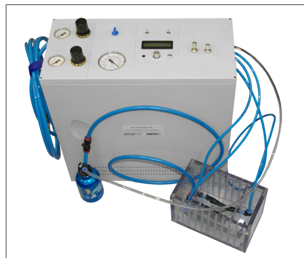
Fig. 4. Lung and heart phantom connected to frontend control device with display
