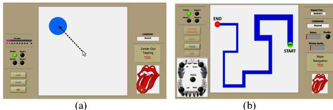
Fig. 6. GUIs for the well-known (a) center-out tapping and (b) maze navigation tasks, similar to what was reported in [8].
