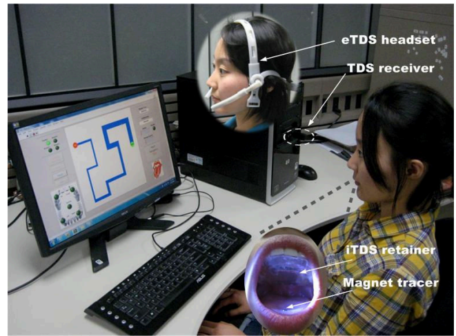
Fig. 5. Test setup for the iTDS dental retainer and the eTDS headset.
