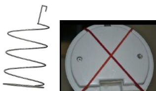
Fig. 3: Wire Frame (left) and lid modification to hold frame (right)
