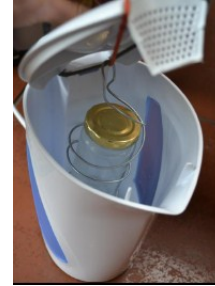
Fig. 1: Photograph of Kettle Heat Treatment System
