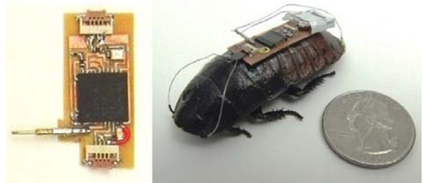
Figure 1: Assembled system-on-chip based backpack with Flexible Flat Cable (FFC) connectors added for battery and probe connections. The system is implanted on a cockroach.
