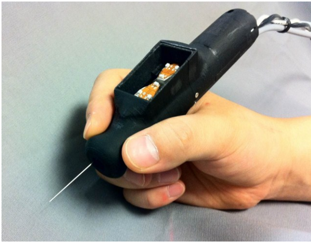
Figure 1. Micron, an active handheld micromanipulator.
