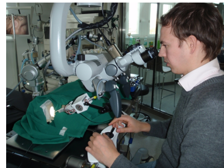
Figure 5: Experimental setup for telemanipulated instrument guidance using a microscope as imaging device.
