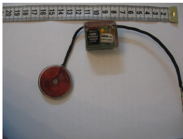
Figure 9. The sealed implantable unit. The small size of the unit makes it appropriate to be implanted in small animals.
