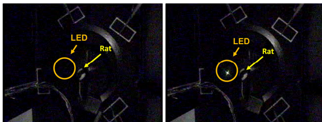
Fig. 5. Detection of the optical marker on the video streaming data.
