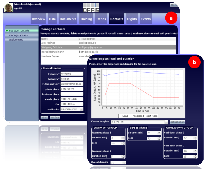
Fig. 4: Screenshots of the PHR: a) Contact details for the alert system, b) Training schedule creation supported by the model for the prediction of the patient's heart rate.
