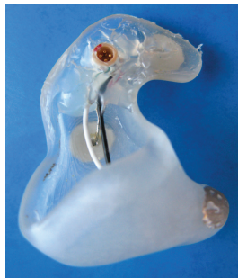
(b) An earplug with electrodes and connector (opposite view of Figure 1(a)). Electrode ERE is visible.
