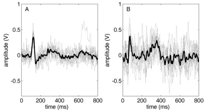
Figure 7. ECG alignment with samples (gray lines) and averaged signal (black line) for S1 (A) and S2 (B)
