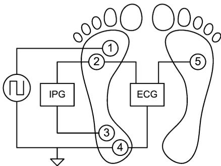
Figure 1. Contact points between electrodes and feet
