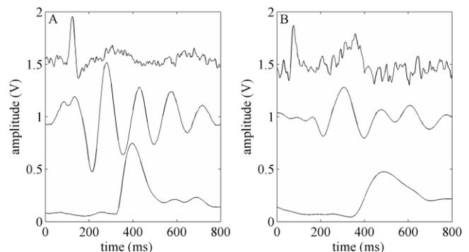
Figure 6. Waveforms obtained after signal processing from S1 (A) and S2 (B): ECG (top), BCG (middle) and IPG (bottom)
