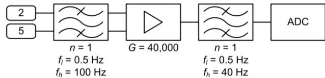
Figure 2. ECG acquisition system
