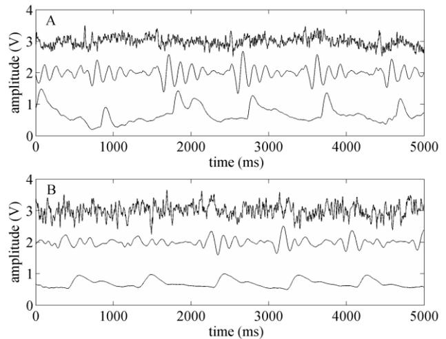
Figure 5. Sample of acquired signals from S1 (A) and S2 (B): ECG (top), BCG (middle) and IPG (bottom)
