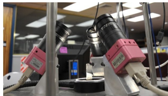
Fig. 1. Three-camera stereoscope fixed in place on solid aluminum blocks.
