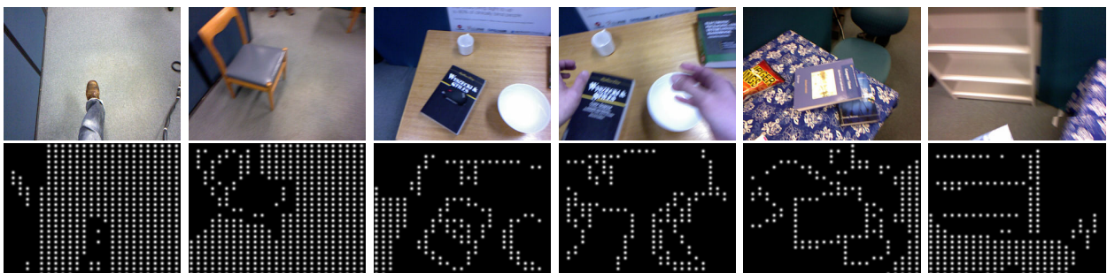
Fig. 10: Free form trial: Subject asked to organise a domestic environment. Top: Kinect colour camera. Bottom: User's POV within HMD (ground plane and structural edge modes). Full Video: http://youtu.be/iK5ddJqNuxY
