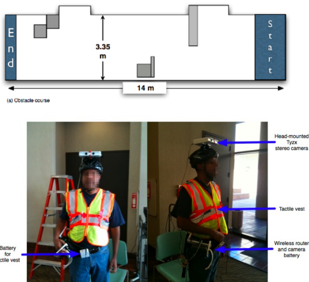
Figure 1 – Top - Overhead view of an obstacle course used for navigation testing. Bottom – The prototype wearable system for navigation.
