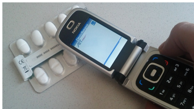
Figure 2. Action of reading data of pill takeout (time and amount) by touching the blister with the NFC enabled mobile phone.
